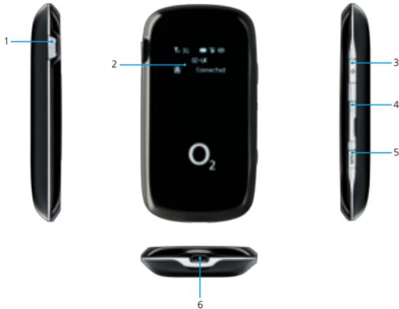
1. Antenna connection (antenna not supplied).
