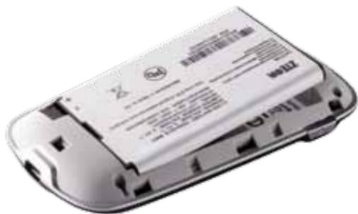
4. Line the battery cover up and press gently to close the case.
