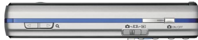
interfering with the lens, flash or, when in video mode, the 3LED video light. When using the camera, the side keys (now effectively on the top of the handset) act as the zoom in/out buttons. There's also a slider switch to alternate between camera, video camera and playback modes. When in camera or video camera mode, keys 3, 6, 9 and # act as shortcut keys to various functions.
